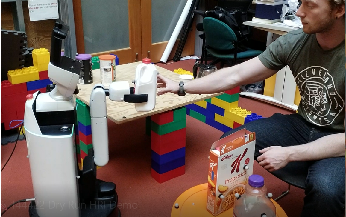
Figure A-1: Pike in action on the Toyota Home Service Robot (HSR). In this image, Pike is assisting a human with a food preparation task. By observing the humans actions and making inferences about their intent, it is able to anticipate items the human will need and retrieve them.
