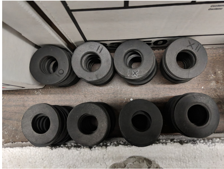
Figure 3.7: Rubber washers were made of 0.3 cm (1/8") thick commercial grade Rubber-Cal Neoprene and were stamped with 5 cm and 2.5 cm diameter leather punches. The labeling of disc identification codes is visible on the top row of rubber washers.
