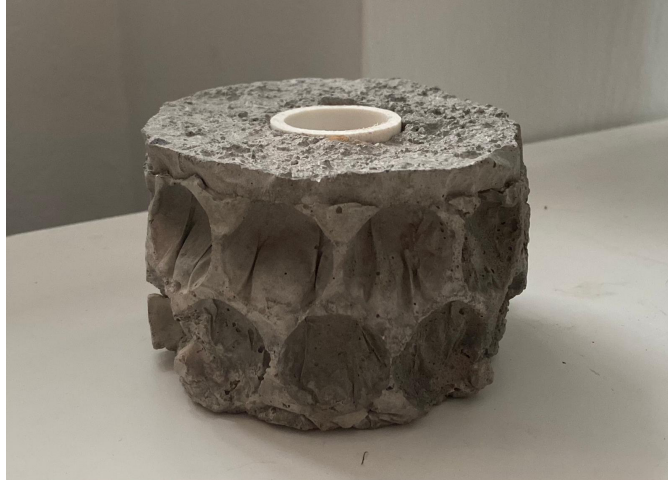
Figure 3.1: The artificial habitat structures are discs with a 6.4 cm height, a 10 cm diameter, and a 3.2 cm diameter center hole. The center hole facilitates deployment by allowing discs to be strung onto ropes, chains, or pipes.
