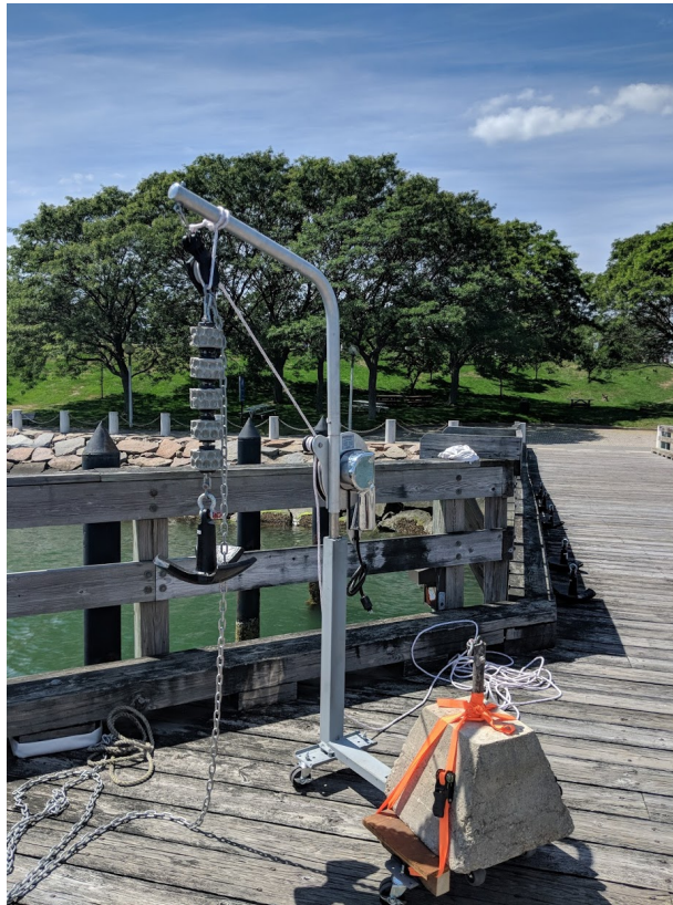
Figure 3.11: The small forklift used to lower and lift hanging research structures from the pier into the water. A 60-kg counterweight was used to balance the forklift.
