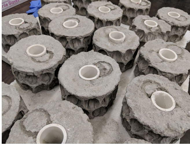
Figure 3.8: Each disc was fitted with 1” nominal PVC pipe through the center hole to prevent damage to the disc via abrasion from the chain.
