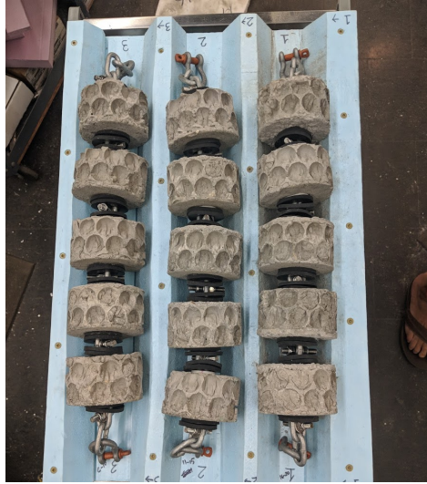
Figure 3.9: Five discs were strung onto each chain segment and fixed in place along the chain with a piece of threaded rod bolted into the exposed chain link above and below the disc.
