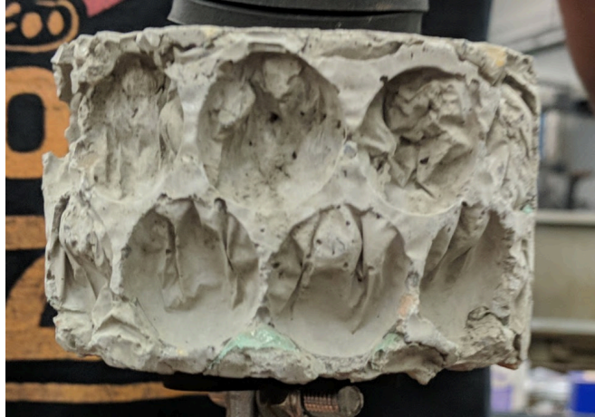
Figure 3.2: The lateral surfaces of the discs are textured to facilitate recruitment of biodiverse growth. The lateral surface of the discs is textured with two rows of evenly spaced hemispherical cavities that are 2.0 cm in diameter, 0.6 cm in depth from the lateral surface, and 0.5 cm apart. The inner surfaces of each hemispherical cavity were further textured with a knife and re-packed with concrete clumps. Additionally, aggregates up to 0.5 cm in diameter in the concrete mixture contributed to a randomly bumpy overall surface texture.
