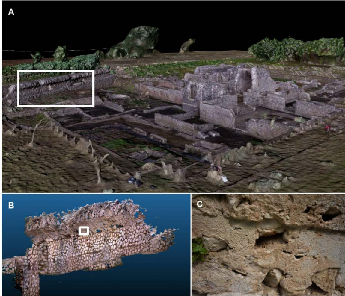
Figure 3-1: Collection location of the ancient Roman mortar samples used in this study. A: 3D reconstruction of the Privernum archaeological site, collected using drone photogrammetry. B: 3D reconstruction of the wall from which the mortar sample was collected, using a DotProduct DPI-8 3D scanner, and C: a higher magnification photograph of the wall surface.
