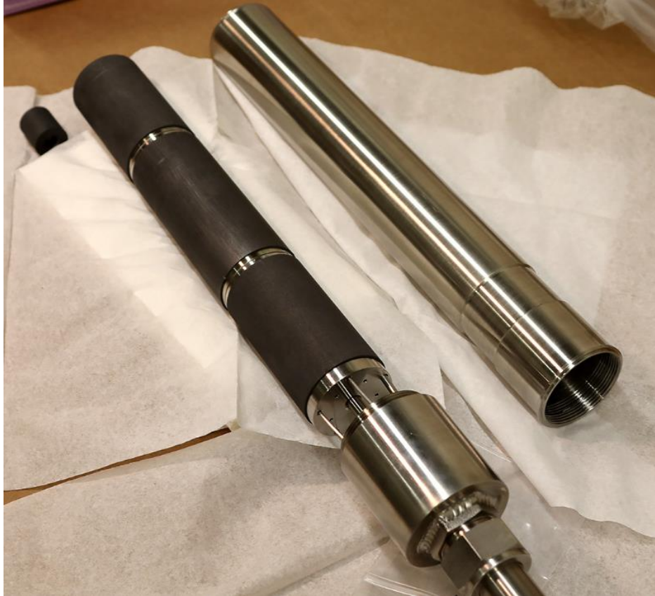
Figure 3.36. Graphite crucibles and nickel capsule cover in an assembly test prior to Flibe filling and the FS-3 irradiation.
