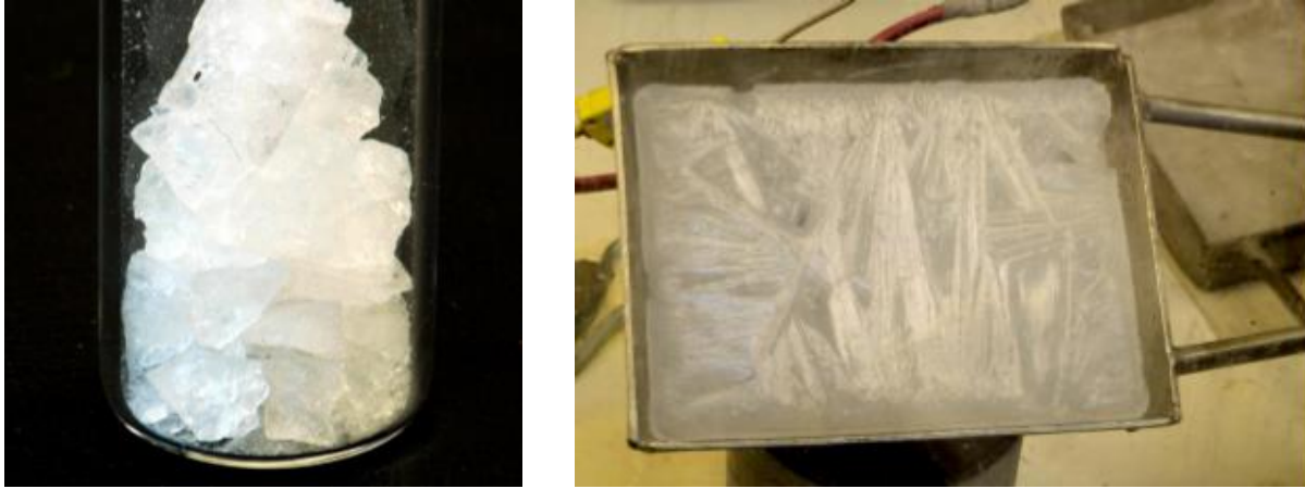
Figure 3.2. FS-1 Flibe (left) and FS-2 and FS-3 Flibe (right) after purification. From [60].
