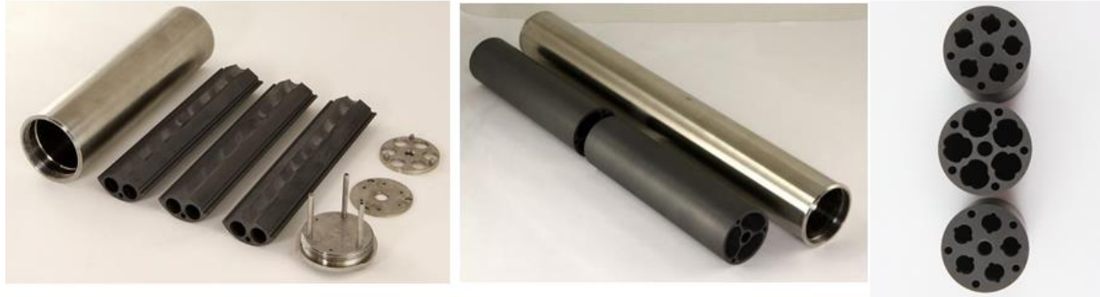
Figure 3.1. FS-1 graphite crucibles (left) and FS-2 graphite (center) along with nickel capsule used for east test. The FS-1 graphite holes are 1 cm in diameter and nickel capsules have similar diameters. Graphite crucibles for FS-3 are pictured on the right. From [17, 145].
