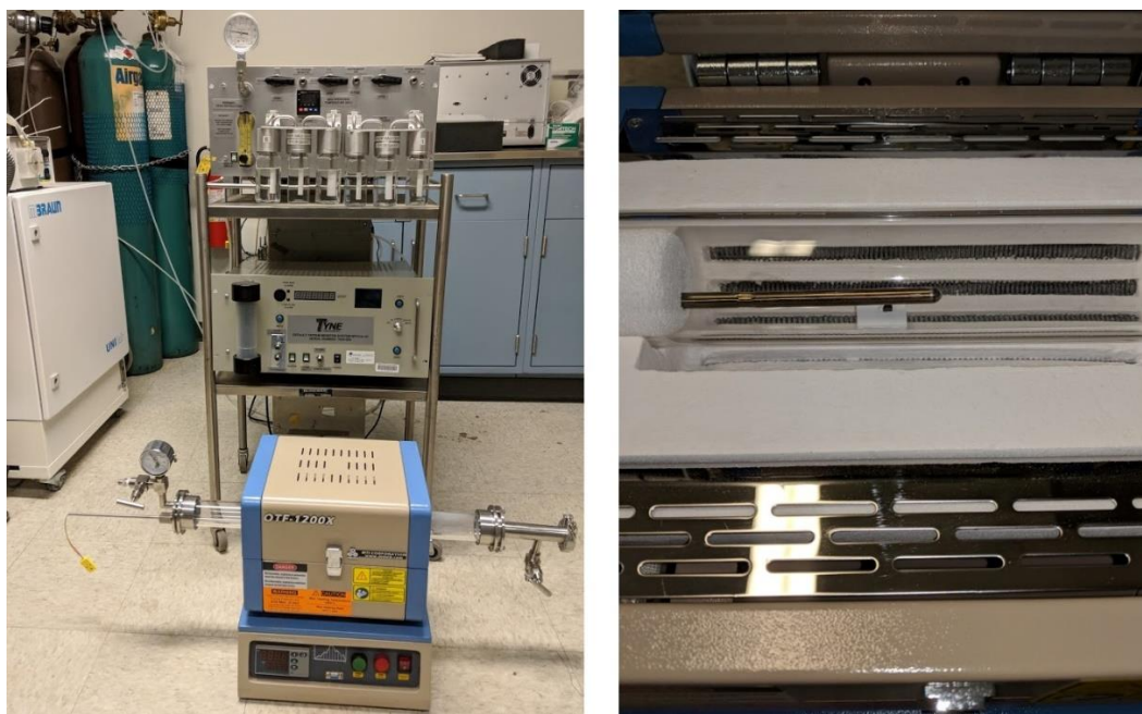
Figure 3.21. Quartz tube furnace with tritium measurement systems (left). Inside the furnace, an Inconel-sheathed thermocouple is positioned through one of the ceramic tube insulators while the samples rest on a high-temperature compatible sample tray in the quartz tube (right).
