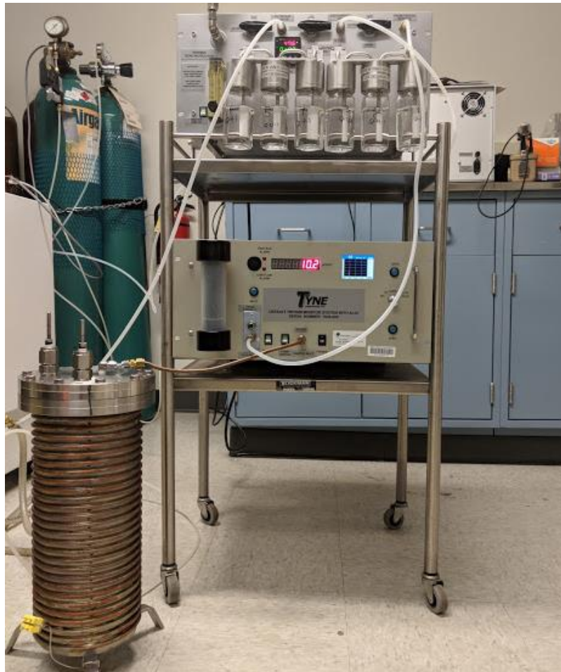
Figure 3.13. Thermal desorption facility used for FS-2 samples. Desorption occurs in the steel vessel furnace, gas flows into the ion chamber, and then tritium is trapped in the water bubbler.
