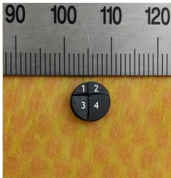
Figure 3.39. Subsection labeling diagram for the FS-3 IG-110 sample U44 from the upper crucible.
