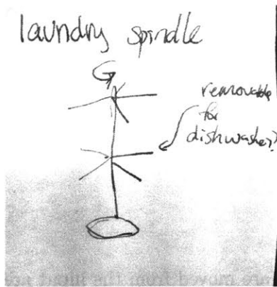
(c) This concept is similar to the laundry spindle. Each level of the arrangement can rotate independently.
