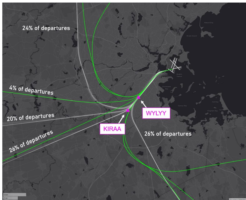
Figure 51. Baseline radar tracks from 2017 (white) are compared to simulated flight tracks of aircraft flying the proposed procedure (green).
