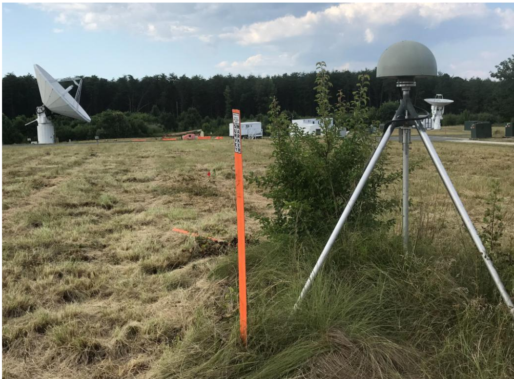
Figure 4: The North GNSS station (GODN) at GGAO with the 12-meter VGOS antenna in the back left.
