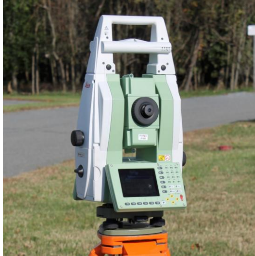
Figure 5: The Robotic Total Station (RTS) at GGAO that is part of the site's Vector Tie System (VTS).
