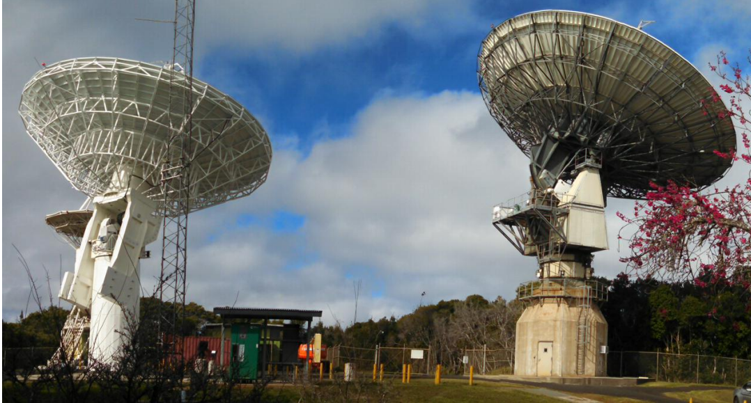
Figure 6: The new 12-meter VGOS antenna at NASA’s Kōke‘e Park Geophysical Observatory (KPGO) on Kauai, Hawaii is shown (left) alongside the legacy 20-meter VLBI antenna (right).
