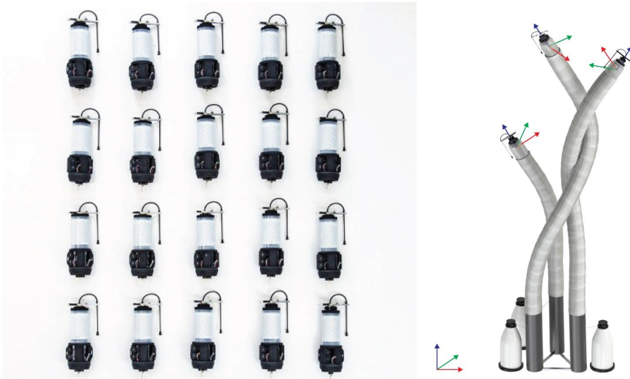
Fig. 5 The photo on the left shows twenty robots. On the right is a rendering of the robots during fabrication with their local coordinate systems relative to the tubes they fabricate, and a global, shared coordinate system that is established during a calibration phase before fabrication begins
