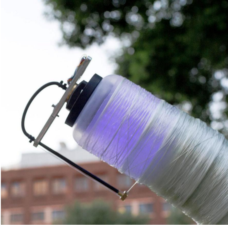
Fig. 3 On the left is a picture of the robot fabricating a section of tube. The majority of the robot is within the tube, with only the wind arm protruding to continue fabrication. On the right are pictures of weaving samples fabricated by the system, adapted from (Blinded). Each is a single segment fabricated independently by a robotic system, not appended onto a tube
