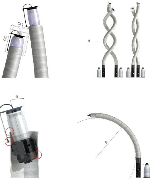
Fig. 9 This figure, originally presented in (Blinded), shows how robot kinematic constraints (on the left) can limit and impact the overall structure (on the right). On the top left, the wind arm and protrusion of the robot forms a collision cylinder with other robots, tubes, and obstacles, and limits how close together tubes can be, shown to its right. On the bottom left, the robot's self-collisions with its own tube limits its tilting capability and hence the overall possible curvature of the tube, shown to its right
