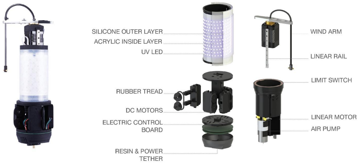
Fig. 1 An exploded view of a single Fiberbot, originally shown in (Blinded). Left, a full image of a Fiberbot. Right, the upper left is the inflatable mandrel, bottom left is the mobile base, top right is the wind arm, and bottom right are internal actuators for the wind arm and mandrel.
