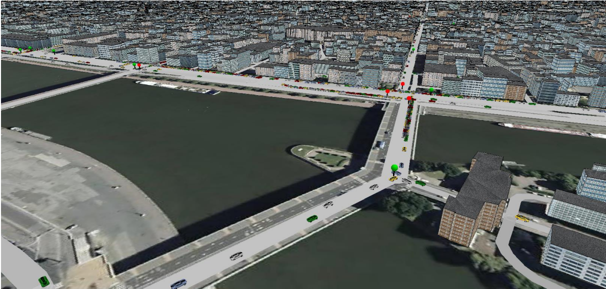
Figure 6. Example of displays that can be defined with GAMA: used of 3D obj files with textures for cars, a geo-referenced satellite image as background, and a building shapefile with 3D extrusion and textures for buildings.
