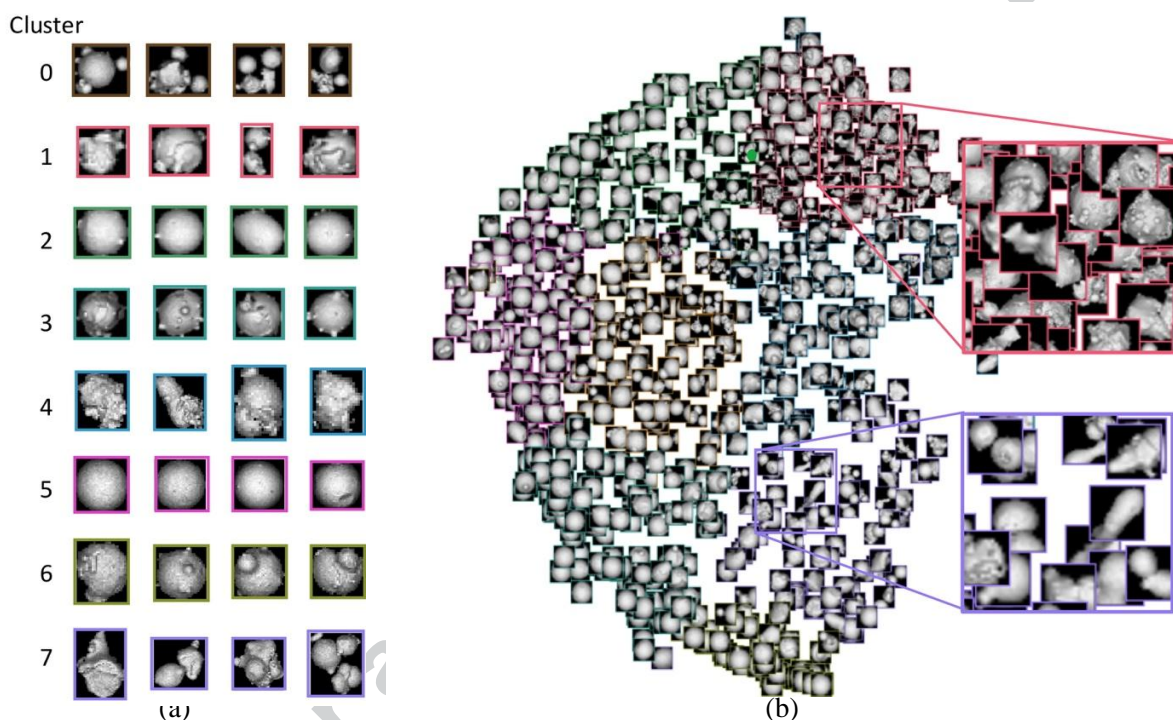
Figure 9. The visual density map for a metal powder. (a) Individual particles are clustered visually; here an 8-cluster k -means analysis showing four example particles per cluster. (b) A t-SNE visual similarity map for about 1100 Inconel-718 particles. Insets show how visually similar particles cluster (red = rough, agglomerated, purple = elongated). Box color corresponds to k -means cluster number. The k -means cluster statistics and image density map are quantitative fingerprints of the powder material.
