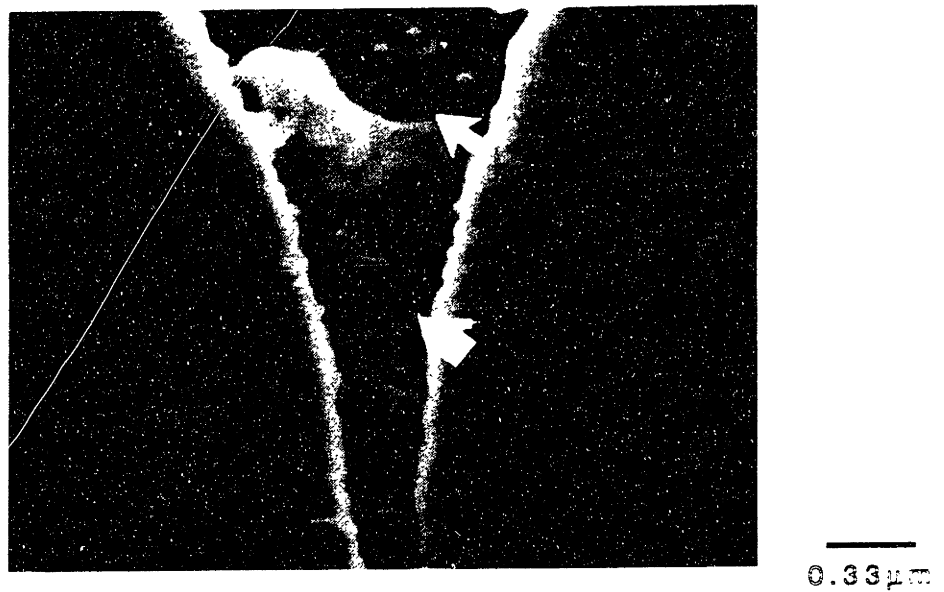
Figure 3.4.4: Secondary electron SEM micrograph showing Fe and Cu-rich intermetallic in narrow interstice of a G/6061 Al MMC after etching (Specimen 8).
