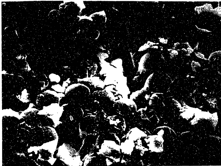
Figure 5.2.6: Secondary electron SEM micrograph for G/Al-5% Zn MMC at high magnification showing discontinuous corrosion product formation after 24 hours in aerated 3.15 wt.% NaCl solution.
