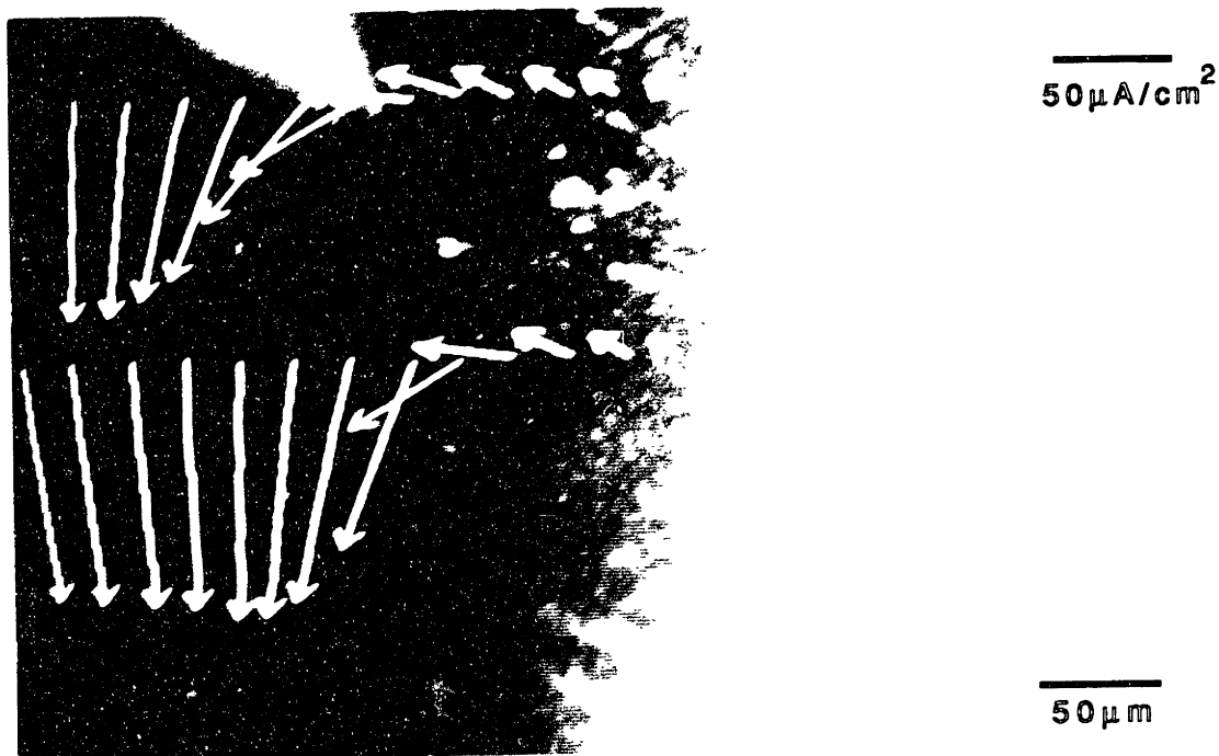
Figure 6.3.7: Video image of an Zn-implanted model G/Al MMC specimen with a 16mm outer Al diameter at time = 48hrs. SPM current density vectors have been superimposed. Solution 0.01 M NaCl open to air. pH~7
