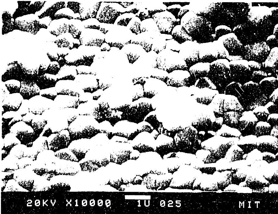
Figure 4.2.9 SEM secondary electron images of MA956 after oxidation at 1200°C for (a) 2hr and (b) 50hr.
