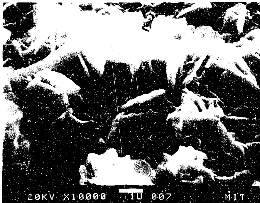
Figure 4.1.9 SEM secondary electron images of APM after oxidation at 1000°C for 100hr. The central particle was identified by EDXA as Zr-rich. The surrounding blade-like oxide structure is indicative of metastable \theta -Al 2 O 3 .
