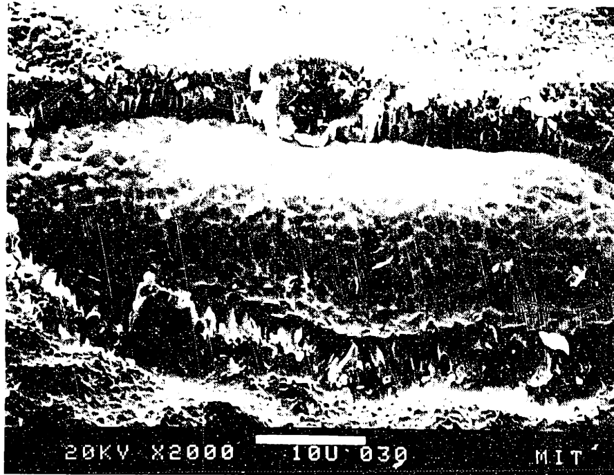
Figure 4.2.7 SEM secondary electron images of APM after oxidation at 1200°C for 100hr. The oxide has spalled away at the edge of the sample revealing the columnar structure of the oxide
