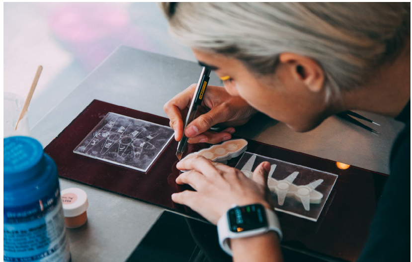
► Figure 21: The part is removed from the mold. The inserts that are designed to create a void are removed. Other inserts such as the adhesive structure wings remain inside the silicone part.
