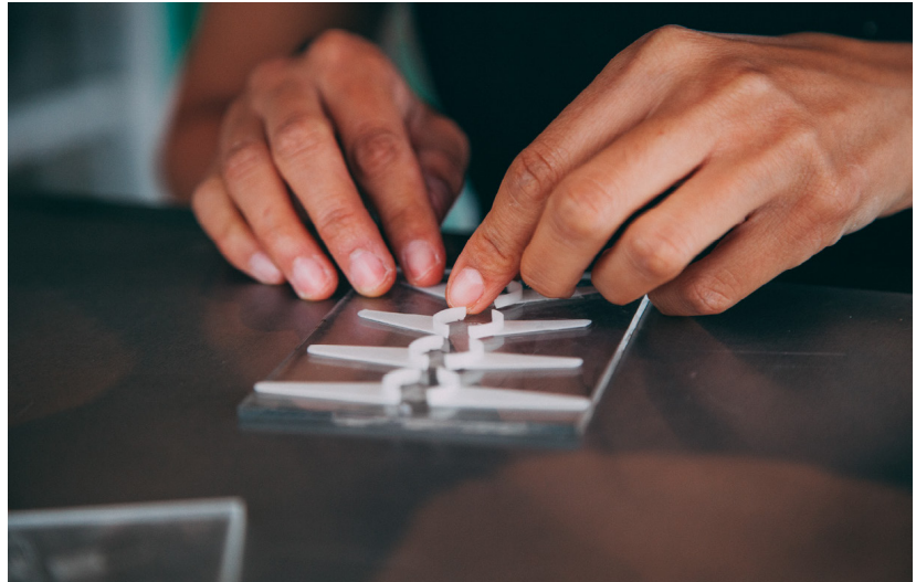
► Figure 18: Inserts are placed and adhered to the acrylic sheet
