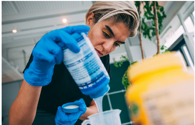
► Figure 19: Part A of the silicone is mixed with the silicone dye. Then Part A is mixed with Part B.
