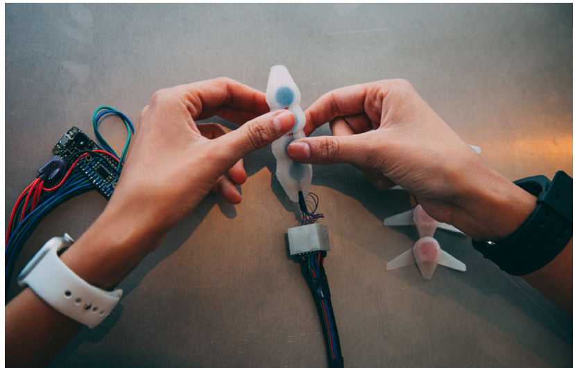
► Figure 22: The actuators are encased in the housing (pictured in blue). Then the assembly of actuators and housing are inserted into the silicone (in place of the inserts that were removed).
