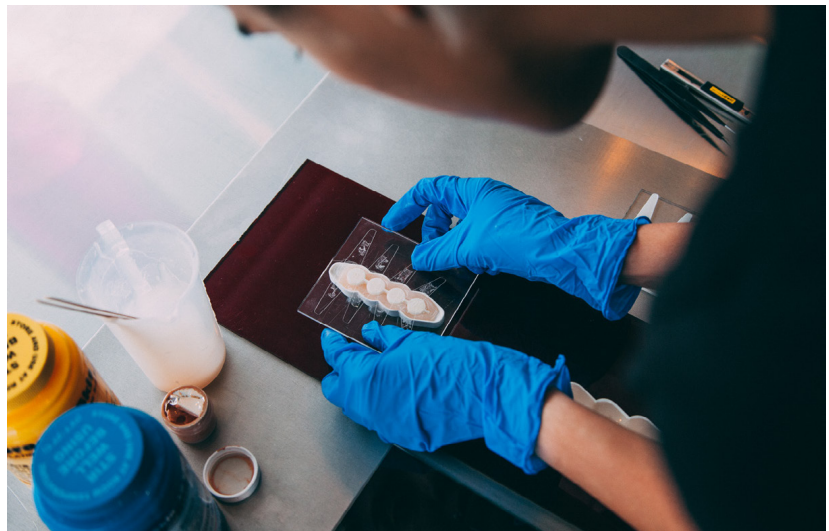
► Figure 20: Silicone is poured into the mold. Then the acrylic sheet with the inserts are inserted into the silicone.
