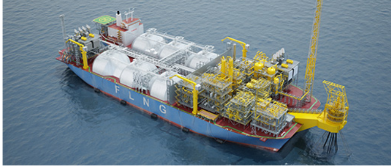
Figure 6-3: Twin-hull FLNG by SBM offshore, from ref[35]
