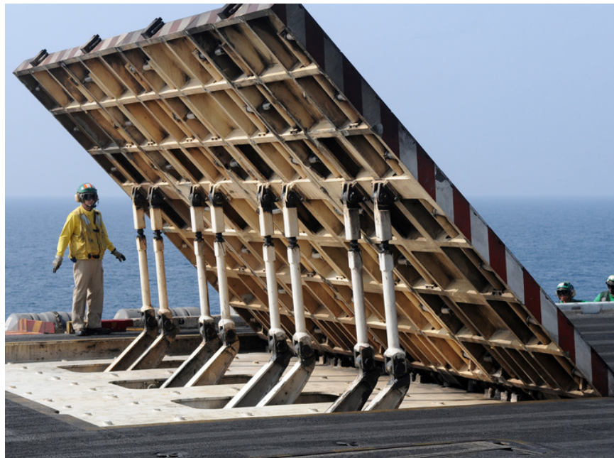
Figure 2-8: Jet blast deflectors, from ref[50]
