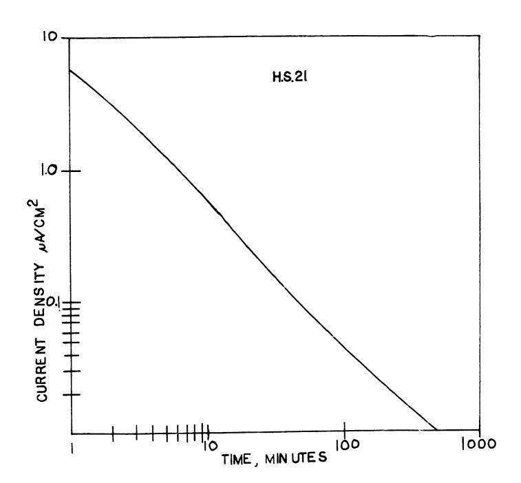
PASSIVE CURRENT DENSITY VS. TIME CURVE OF M.I.T. ALLOY NO. 7 IN 0.9% NaCI SOLUTION
