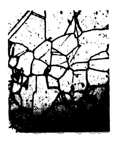
Figure 19 M.I.T. Alloy NO. 7. Annealed at 1200°C for 4 Hours. and Quenched in Water. 5% HCI Electrolytic Etch. X500.
