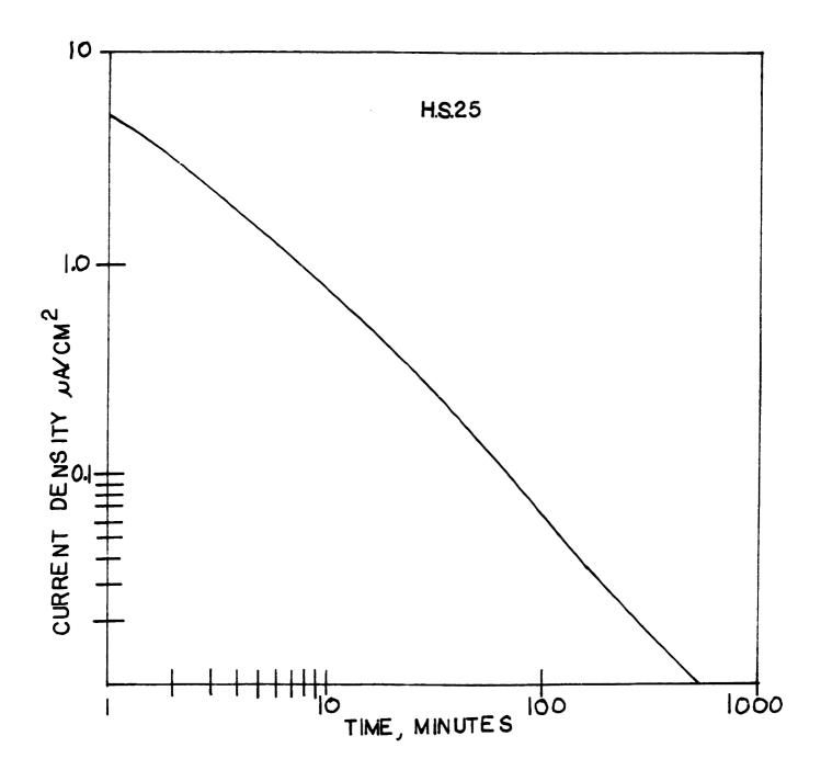
PASSIVE CURRENT DENSITY VS. TIME CURVE OF HAYNES STELLITE 21 IN 0.9% NaCI SOLUTION
