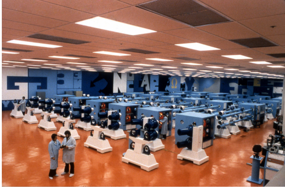
Figure 2-14: The 24-beamlines of the Omega facility at LLE [55]
