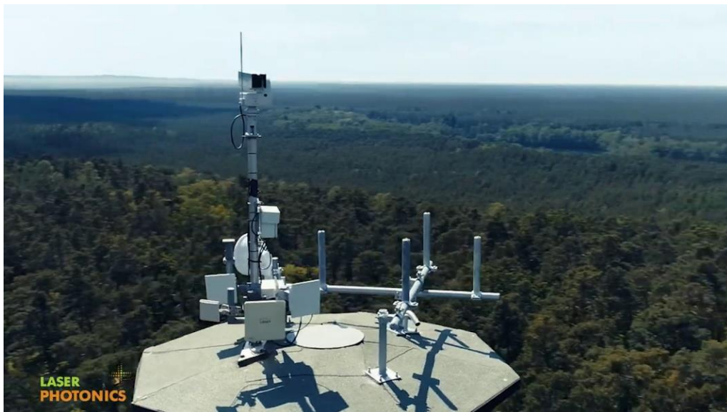
Figure 3-5: A wireless computer vision-based fire detection system by IQ FireWatch [148]
