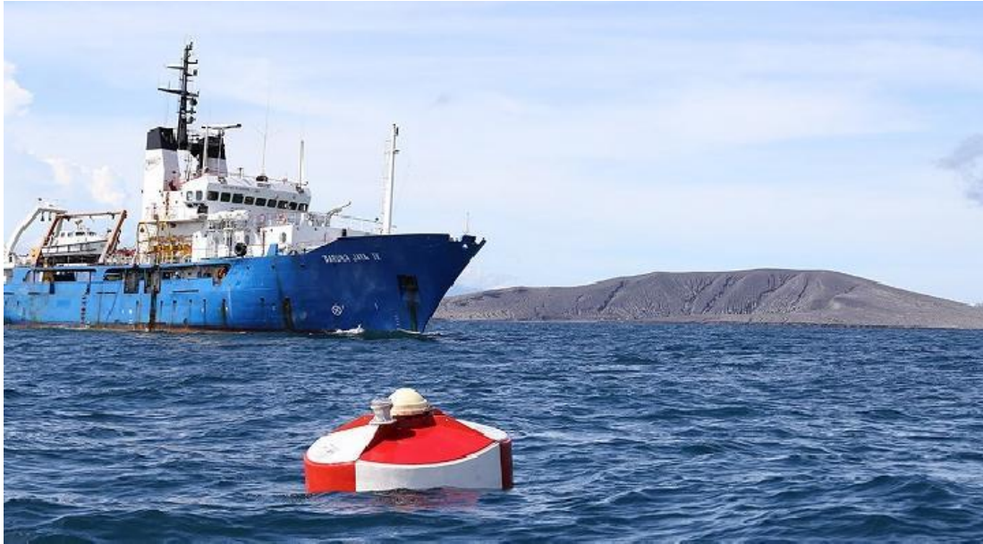
Figure 3-11: BPPT's tsunami surface buoy with its Iridium antenna [154]
