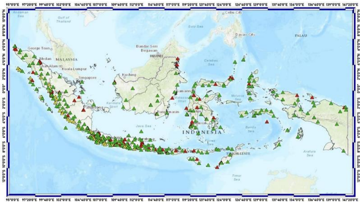
Figure 2-9: InaTEWS' network of accelerometers and intensity meters [29]
