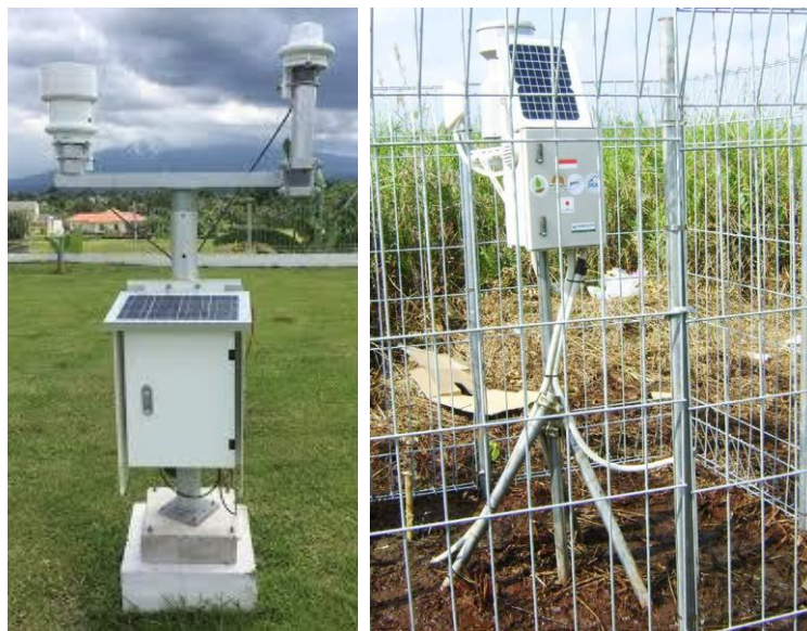
Figure 3-10: BMKG's automatic weather station (left) [153] and BRG's peatland water level monitoring system (right) [76]
