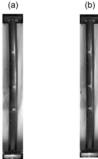
Figure 12 Video processing. Snapshot of the magnified videos with frequency peak 1 a and 3 b . For the peak 1, the magnification frequency band is 42Hz-46Hz and amplification factor 100. For the peak 3, the magnification frequency band is 148Hz-152Hz and amplification factor 300
