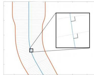
Figure 15 . Flight track (in blue) with a noise contour (in red) molded around it, from [5].
