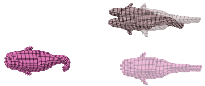
Fig. 9. “Closed-loop co-optimization” experiment: Performances of the initial (top) and the optimized geometric design (bottom) of the swimmer. The color of the swimmer is interpolated with their weights \alpha from the base shapes’ colors in Fig. 5. The design is simulated to swim forward from an initial position (transparent) on the right. The swimmer’s final locations after a fixed amount of time are rendered as solid meshes. A longer traveling distance is preferred in this experiment.
