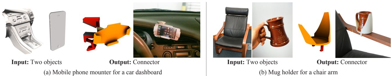
Figure 1: AutoConnect creates 3D-printable customized connectors based on shapes of two given objects and a user-specified configuration. Custom holders are created for connecting a mobile phone to a car dashboard (a), and a mug to a chair (b).
