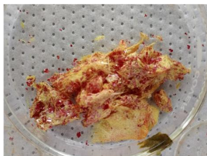
Figure S6. Picture of n = 2 BA-MAPbI crystals with yellow, needle-like crystal by-products.
