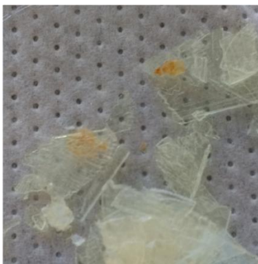
Figure S10. Orange coloring on white crystals of n = 1 BA-PbBr. Because the synthesis of n = 1 BA-PbBr does not involve MA cation, these orange colorings are not believed to be due to the formation of bulk MAPbBr 3 or higher members of bromide 2D LHPs.
