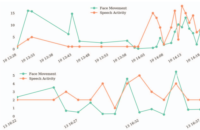
Fig. 3: Example data collected and processed by the Analytics Engine for two 3-person face-to-face remote meetings with the custom WebRTC platform. Face movement indicates the average absolute change of tracked facial points for each participant. Speech Activity is the number of utterances spoken by group members. Values are binned and averaged for each minute of the meeting.
