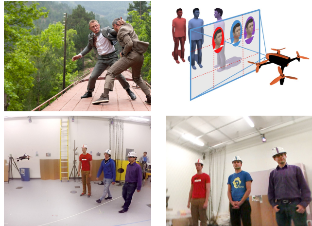
Fig. 1: We propose a real-time method to film shots of dynamic scenes automatically. The user specifies target positions on screen. We solve for robot trajectories and gimbal controls, producing footage that adheres to aesthetic constraints, minimizes visual occlusion and produces collision-free trajectories in dynamic scenes.
