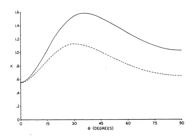
value of k is on the order of unity for all lamina angles, but varies by a factor of two to three, depending on the material, as 9 varies from 0° to 90°. The variation is more severe for NARMCO 5505, which has a maximum k of 1.58 at 35.5°, than for Morgenite II, which has a maximum k of 1.13 occurring at 29°. Since k is basically a function of the material properties, it does not go to zero at 0° or 90° even though the in-plane and interlaminar shearing stresses vanish at these orientations.
