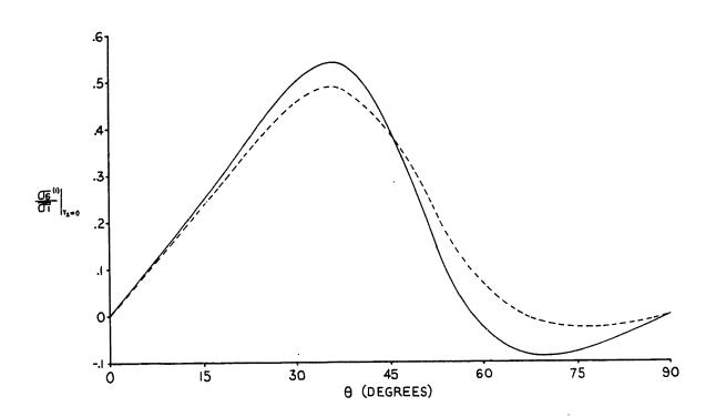
Physically, this behavior results from the fact that angle plies oriented at angles less than the zero edge effect angle attempt to align themselves with the 0° direction, while those oriented at angles greater than the zero edge effect angle attempt to align themselves with the 90° direction, when the composite is placed in longitudinal tension or compression.
