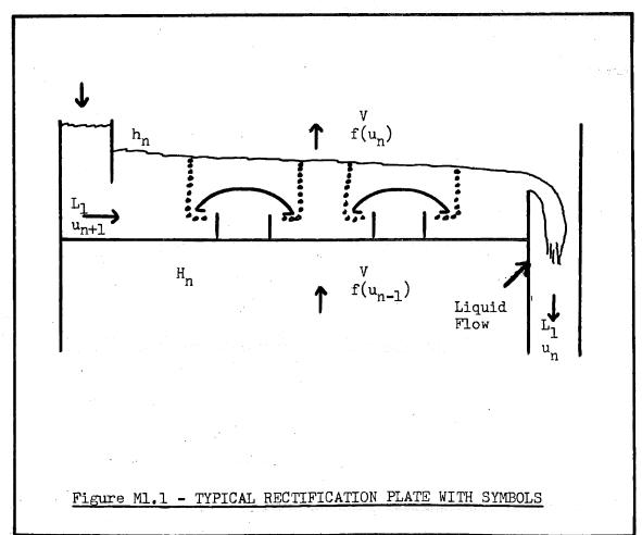
The mass balance of the lighter component in the liquid phase gives equation M1.2 for the upper section and M1.3 for the lower section. The steady-state portions of these equations are seen to be equivalent to the discrete-plate steady-state equations in Figure I2.3.
