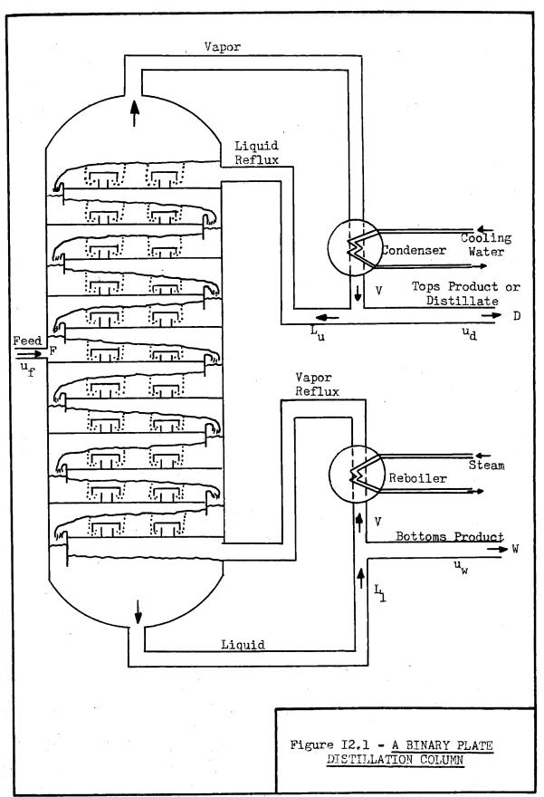
of the column is divided into that portion removed as bottoms product and that portion which is vaporized in the reboiler and fed back to the bottom plate. The other auxiliary equipments, such as pumps to circulate the fluid, valves for control, structural supports, and many others, are not shown in Figure I2.1 but are, nevertheless, essential to the operation of the system.
