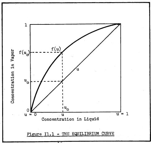
In Figure II.1 the curved line (equilibrium curve) represents a graphical plot of equation II.2. If the relative volatility is not assumed to be constant, then this curve may have a significantly different shape and be represented by a different functional relationship. In trying to understand the meaning of the equilibrium curve it is helpful to consider a point u<sub>0</sub> in Figure II.1.
