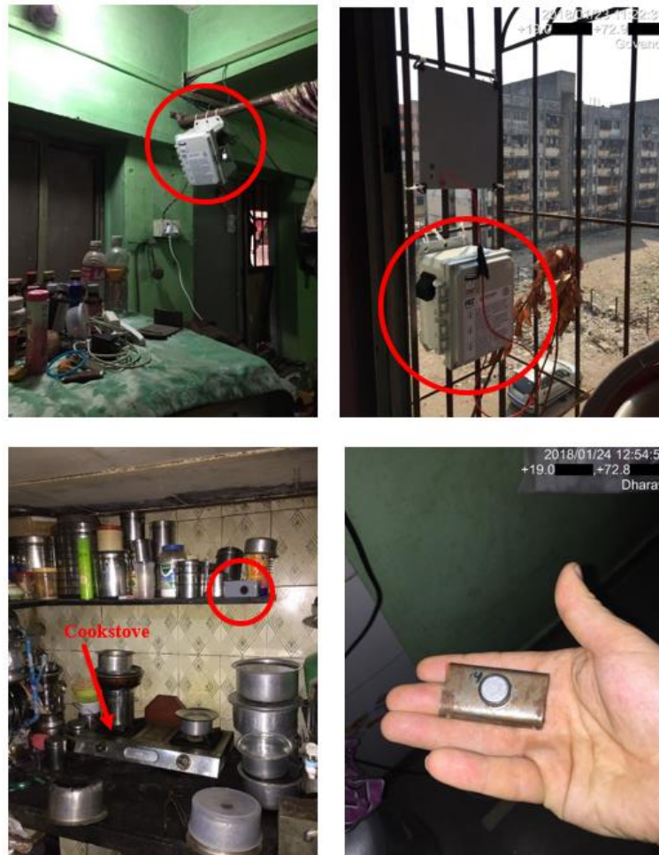
226 227 Figure 3. Examples of pollution logging sensor installations (encircled in red) for indoor and ambient 228 air readings. Top left and right: custom assemblies incorporating Alphasense OPC-N2 optical particle 229 counters (logged measurements). Bottom left: custom assemblies incorporating Plantower PMSA003I 230 PM 2.5 sensors (logged measurements). Bottom right: iButton DS1922L temperature sensors to track 231 stove usage patterns. 232
