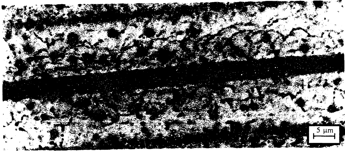
Figure 5.1.13 Decorated, pinned dislocations in the plastic zone surrounding an alumina fiber in an AgCl matrix. Due to the stress from the fiber, some dislocations are bowed. The fiber is out of focus, being a few microns off the image plane.
