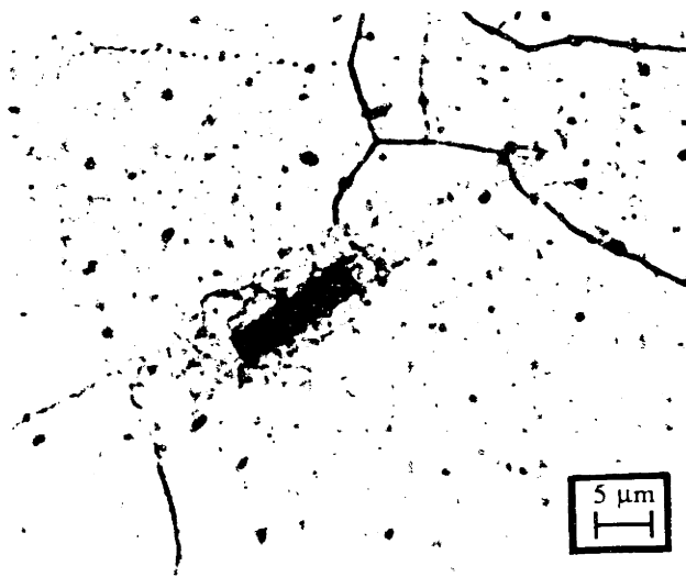
Figure 5.1.14 Decorated rows of prismatic loops punched from a short alumina fiber in an AgCl matrix. After bursting through a subgrain boundary (dark continuous line), the loops change orientation in the second subgrain. Partially resolved dislocation tangles are also decorated around the fiber.
