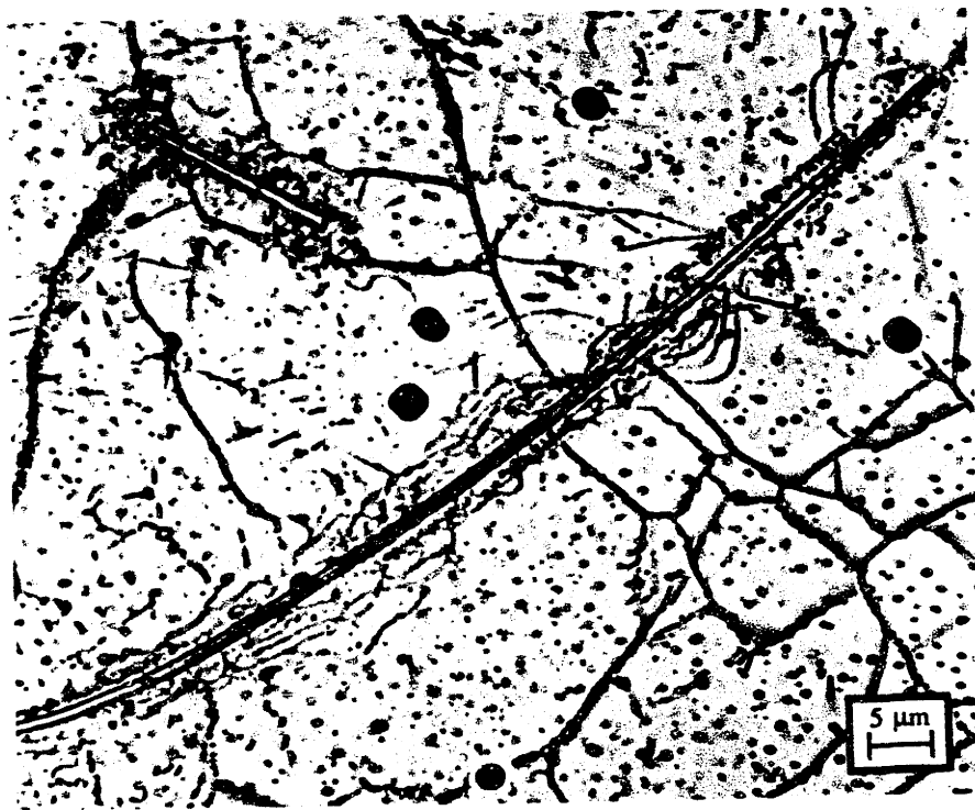
Figure 5.1.26 Decorated dislocations forming the plastic zone surrounding a long glass fiber in AgCl. Some of the dislocations can be resolved.
