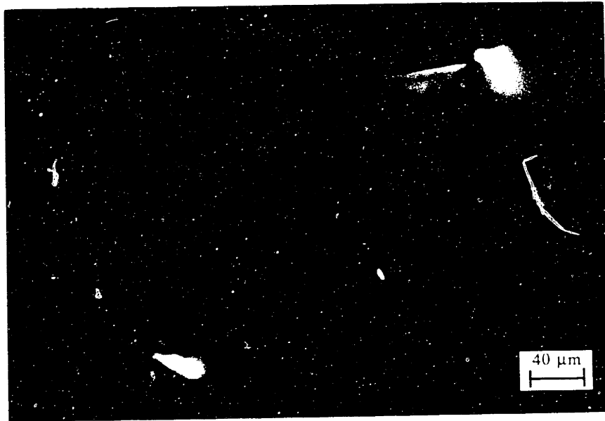
Figure 5.2.3 Stress concentration at the tip of alumina fibers 20 \mu\text{m} in diameter embedded in AgCl (cross-polarized filters used).
