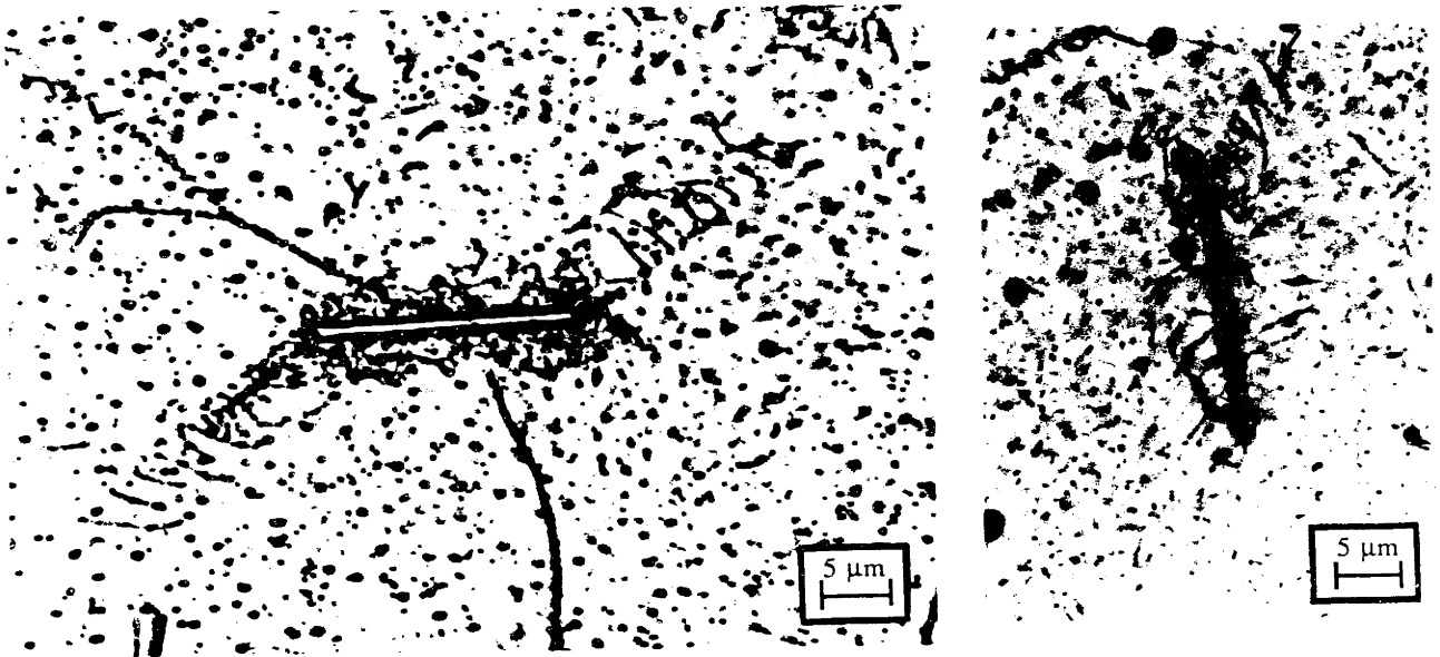
Figure 5.1.19 Glass fiber in AgCl with decorated dislocation structure consisting of two rows of elongated loops emitted sideways at the fiber ends and a plastic zone surrounding the fiber (dislocations are not resolved). The linear feature is a subgrain boundary.
