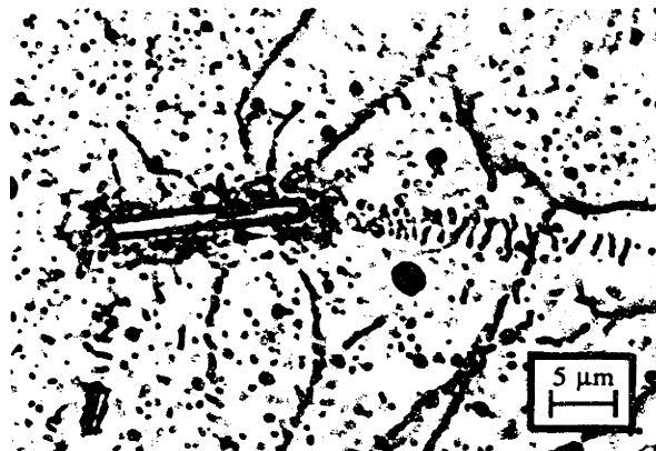
Figure 5.1.18 Glass fiber with emitted row of prismatic loops punched at an angle in AgCl. The fiber is also surrounded by a plastic zone formed of unresolved dislocations.
