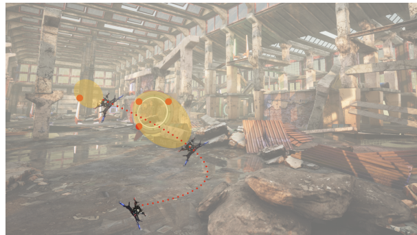
Fig. 1: In the figure above, the desired translational path is shown using the dotted line and the landmarks are depicted using red dots. The field of view is shown by the yellow ovals.
