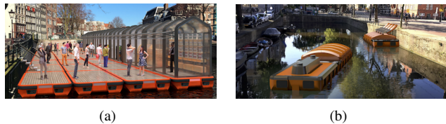
Fig. 1. Concept of autonomous connected-vessels (Roboats): Individual units can (a) tessellate together to form floating stages and public squares on waterways and (b) serve as floating garbage bins that autonomously transfer waste.
