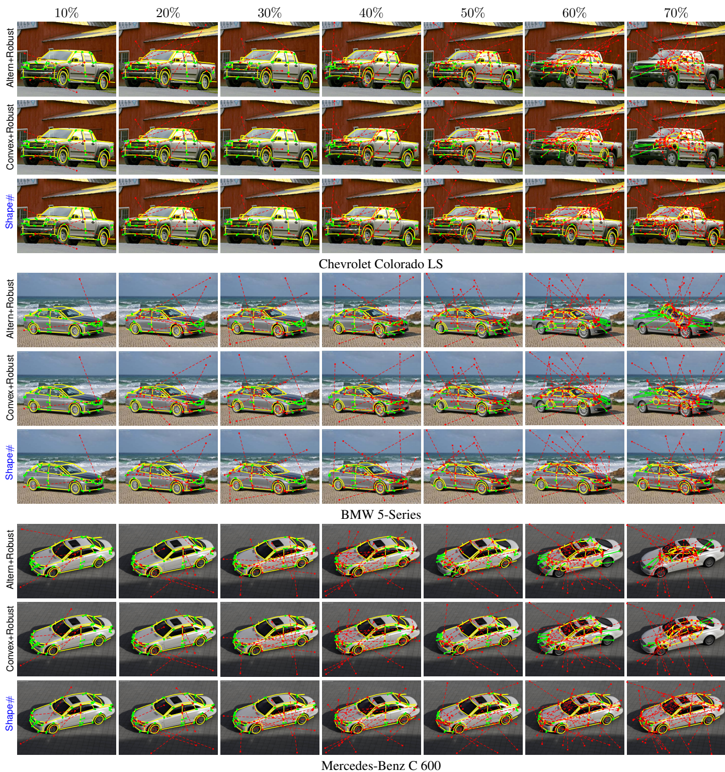
Figure A2: Qualitative results on the FG3DCar dataset [26] under 10 – 70% outlier rates using Altern+Robust [50], Convex+Robust [50], and Shape#. Yellow: shape reconstruction result projected onto the image. Green: inliers. Red: outliers. Circle: 3D landmark. Square: 2D landmark. [Best viewed electronically.]
