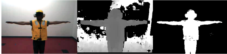
Fig. 2. Example images of input image (left), depth map (middle), and mask image (right). The “T-pose” shown in the figures is used for body tracking initialization.
