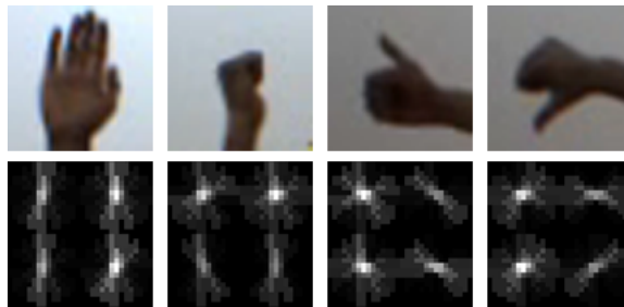
Fig. 6. Four hand poses and a visualization of their HOG features. Bright spots in the visualization indicate places in the image that have sharp gradients at a particular orientation, e.g., the four vertical orientation in the first visualization.
