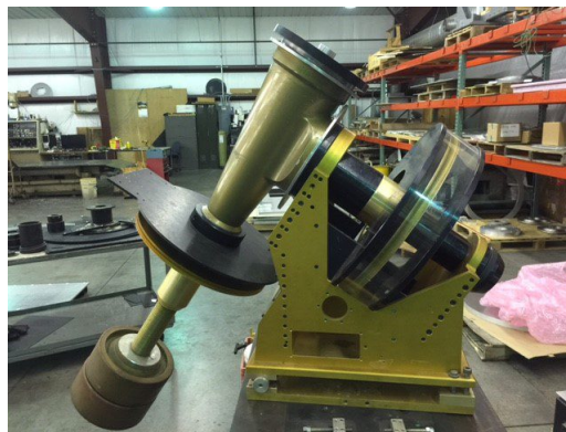
Figure 8: Custom tracking mount by Optical Mechanics, Inc
