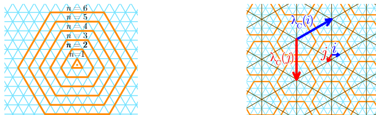
Fig. 14: Left: Scaling \mathcal{C}_n cell shapes; they are the concentric balls, in \mathbb{T} , centered on the vertex at the center of the triangles of \mathbb{T} . Right: the cells at scale \mathcal{C}_n (in orange) and the underlying rotated triangular lattice (in brown), by -30^\circ , whose vertices are located at the center of the triangle at the center of each cell in the original triangular lattice (the orange dot in the figure to the left).
