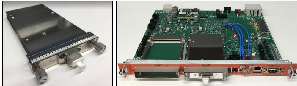
Figure 1. (left) Acacia AC100M CFP optical transceiver module; (right) AC100M optical transceiver assembly with AC100M integrated on ATCA evaluation board.
