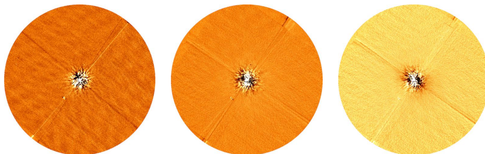
Figure 3. Results of KLIP algorithm applied to each dataset. From left, figures show results for WFE cutoffs of 115 nm, 120 nm, and 130 nm for 20 KL modes. KLIP was applied with 1 annulus and 1 subsection, but streaking in each frame led to the apparent quadrants in the output images. The ghost spot is visible in the lower left corner of each image. These results show how the KLIP algorithm handles data with different levels of WFE and noise.
