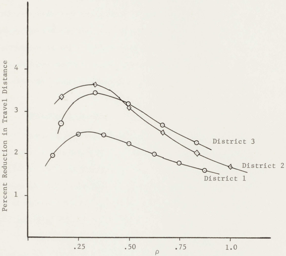
FIGURE 3.13. Percent Reduction in Average Travel Distance Using Call Location Information. Hypothetical Districts 1, 2, and 3.
