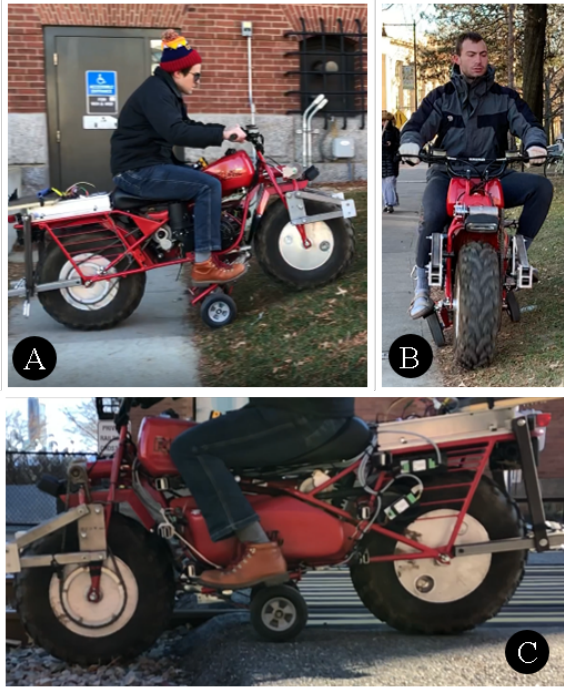
FIGURE 10. DEMONSTRATIONS OF THE BALANCE BOARD BEING OPERATED ON UNEVEN TERRAIN. (A) Steep uphill slopes, (B) side slopes, and (C) going down curbs in changing terrain.
