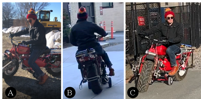
FIGURE 8. IMAGES FROM TESTING THE VEHICLE IN DIFFERENT TURNING SITUATIONS. (A) Putting your foot down for an extremely tight turn, (B) Leaning during high-speed turns, and (C) Tight turns on slopes with both feet on the balance board.
