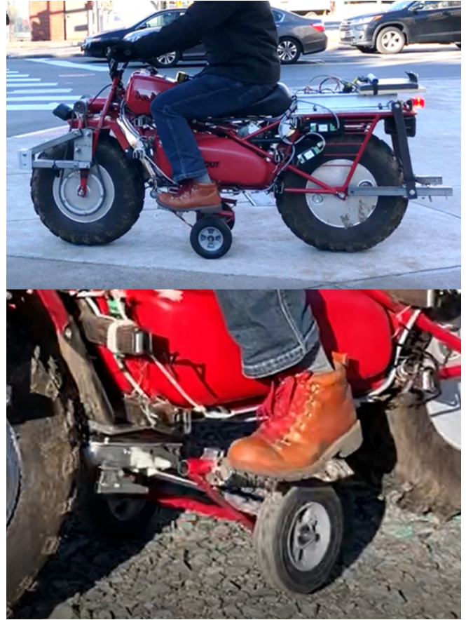
FIGURE 3. THE RIDER STEPS ON THE BALANCE BOARD TO PROVIDE SELF-POWERED ROLL STABILIZATION, ALLOWING THEM TO REMAIN UPRIGHT EVEN AT A STANDSTILL AND NAVIGATING UNEVEN TERRAIN SLOWLY.
