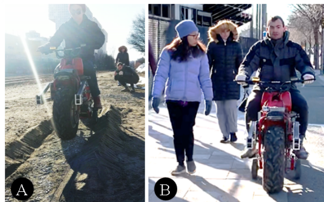
FIGURE 9. EXAMPLES OF SLOW SPEED DRIVING IN TIGHT SPACES. (A) the vehicle travels between dirt mounds separated by 60 cm, the tightest crop spacing it is expected to operate in. (B) the motorcycle is driven at walking pace in a straight line.
