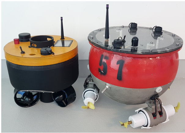
Fig. 3. The two robotic platforms: the new buoy design v2 (left) side by side with one of the previous buoy model v1 (right).
