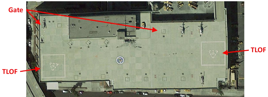
Fig. 5. Los Angeles Hooper Heliport displaying attributes of a “pier” topology. Map © 2018 Google
