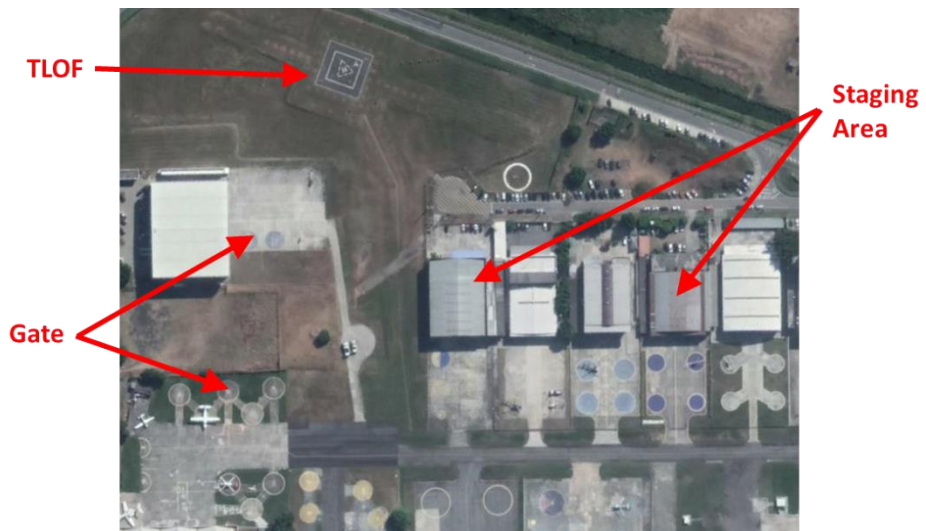
Fig. 6. Aeropuerto Campo de Marte displaying attributes of a “remote apron” topology. Map © 2018 Google. © 2018 DigitalGlobe.
