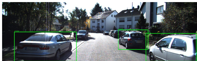
Fig. 3: Object detections from MobileNet-SSD on KITTI sequence 5.
