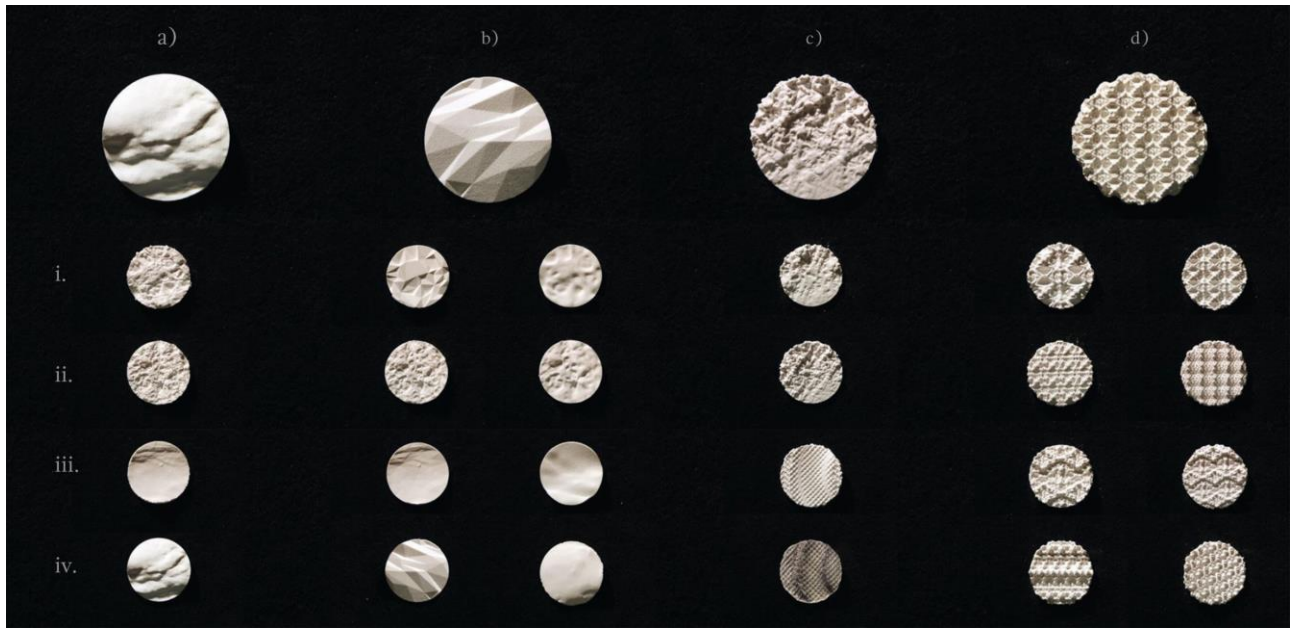
Figure 6: Variations created from prototype 3D texture design tool: a) Sample: a cropped extract of an oyster shell. b) Filter: a mesh-reduce operation and mesh smoothing operation c) Mix: a mathematical z-distortions applied to textures) Loop: tiling of sample textures achieves scalar-manipulations
