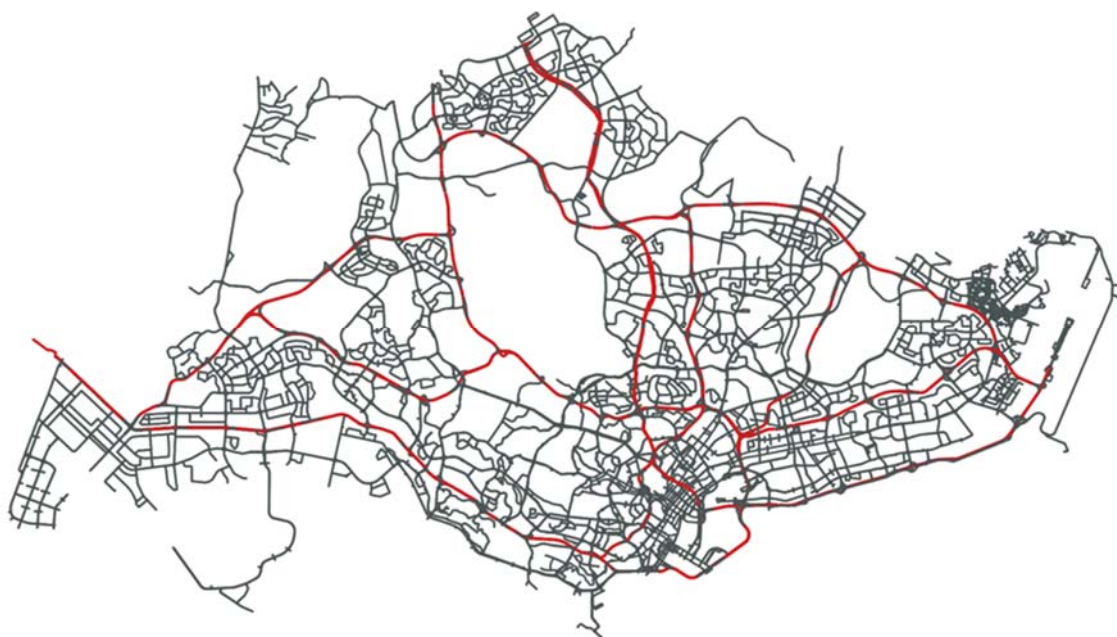
Figure 2. 2030 Singapore road network (red: highway; grey: arterial).
