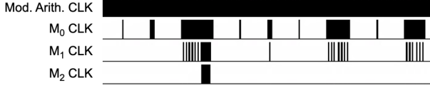
Fig. 5. Simulated waveforms showing memory clock gating in pairing crypto-processor during a snapshot of the final exponentiation computation.
