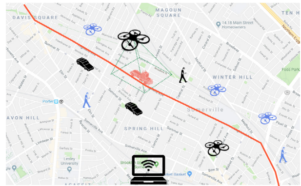
Fig. 1. Example of processing network : smart sensors (in blue and black) collect, process, and communicate data to track the state of a vehicle (in red) in the presence of communication and computation latency.
