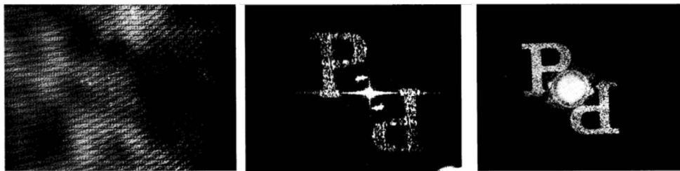
Fig. 1. (a) Detected hologram, (b) Computed image, (c) Optically obtained image. Reproduced from J. W. Goodman and R. Lawrence, “Digital image formation from electronically detected holograms,” Appl. Phys. Lett. 11 , 77–79 (1967), with the permission of AIP Publishing.
