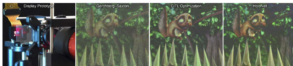
Fig. 21. Conventional computer-generated holography algorithms, such as Gerchberg-Saxton, suffer from artifacts. Recent advances in machine-learning-enabled holographic displays, such as camera-in-the-loop (CITL) optimization strategies [201,202] and neural networks, such as HoloNet [201,202], achieve unprecedented holographic image quality and real-time framerates. Image adapted from [200].
