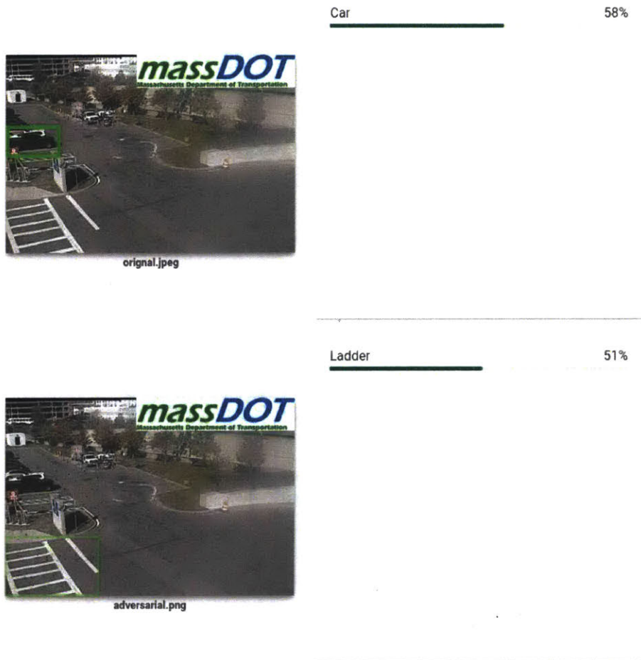
Figure 1-2: Successful demonstration of an adversarial attack on GCV using a traffic-cam image from Massachusetts Department of Transportation
