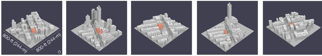
Figure 3.2: Rendered examples of the Radiance scene created for each floor’s daylight simulation. Each scene is about 800-ft by 800-ft (244-m by 244-m), roughly the size of a Manhattan block, with the building in the center. Renderings created using Radiance objView program.
