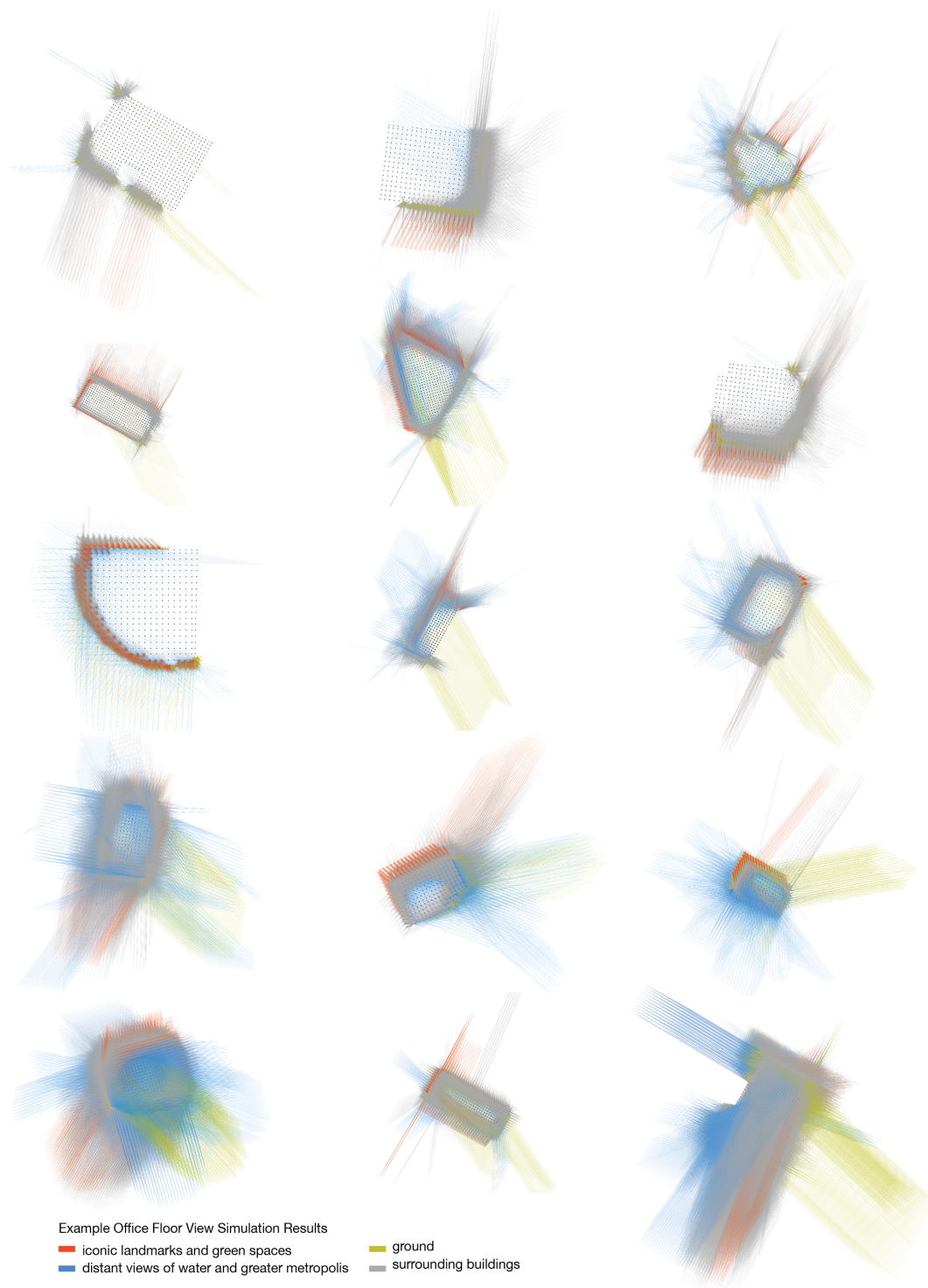
Figure 5.12: Visualization of view simulations on 15 office floors in plan view. The rays shown are at points that meet the 3% MVP requirement; if a point has no rays, it does not meet the MVP limit. The color of each line indicates what view object it intersects. The length and direction of each line indicates which way and how far it extends. The rays have been scaled down by 1/50 . The address, floor number, rent value, sDA, sVA are listed in Figure 5.13.
