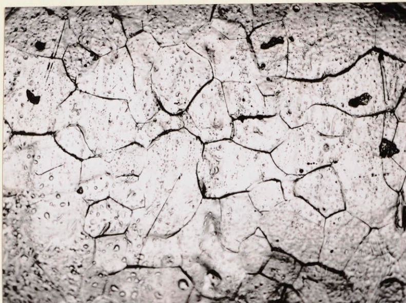
Figure 66. Specimen No. 58 High Purity fine grained aluminum - 0.25-inch part of the specimen. 500° F - Calculated reduction of area= 0.5 percent. 150 x.
