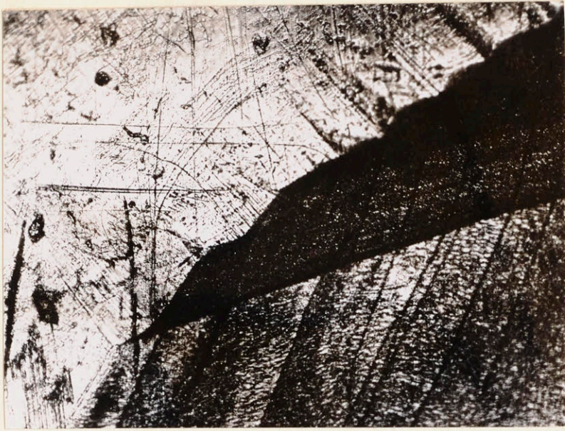
Figure 44. High Purity Aluminum - Coarse Grained - Specimen No. 82. 1100° F - Rupture time = 3.66 hours - 0.25 inch part of the sample 150× (oblique illumination).
