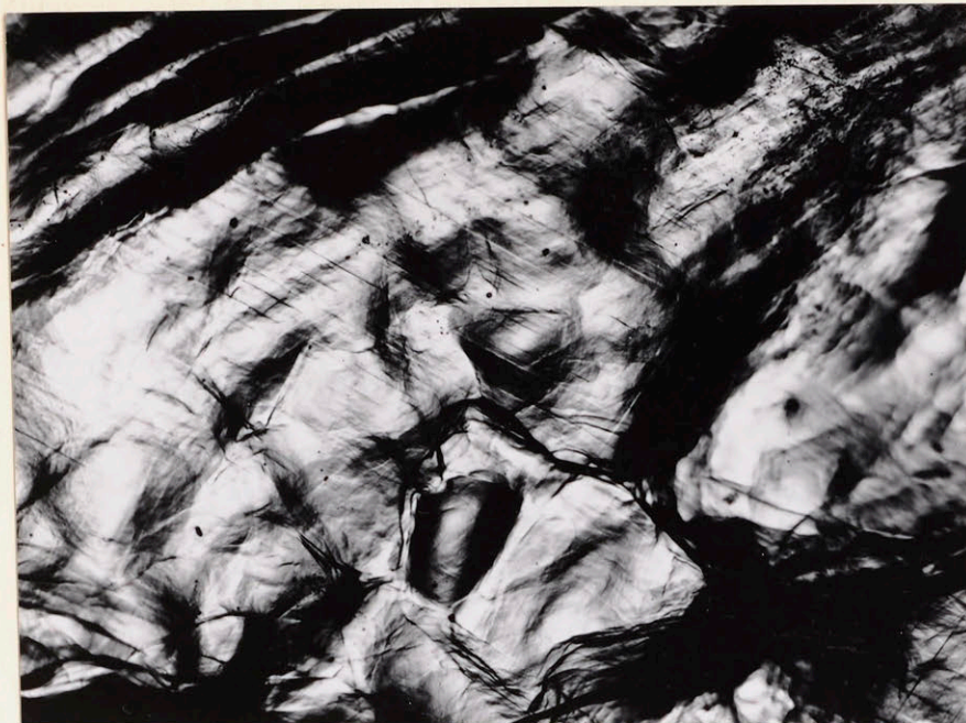
Figure 63. Specimen No. 23 (Point No. 18 of Figure 46). High Purity coarse grained aluminum. R. A. 40 percent. 700° F, 13.5 hours estimated rupture time. 150 x.
