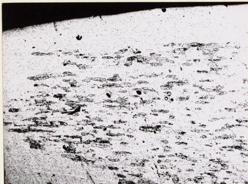
Figure 77. Longitudinal section of specimen No. 224 (Point No. 6 of Figure 70) 2S aluminum. 1100° F, 0.78 hour rupture time. Near neck. Electrolytic polish and etch. 50 x.
