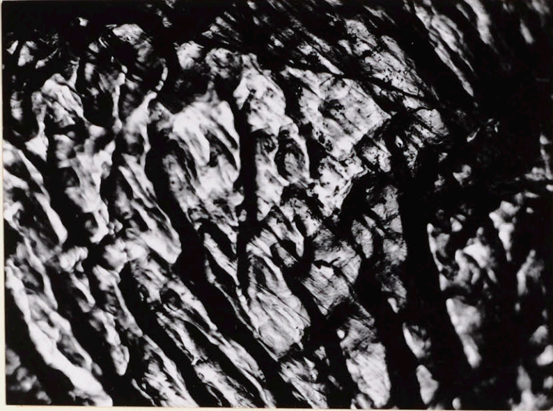
Figure 57. Specimen No. 89 (Point No. 6 of Figure 46). High Purity coarse grained aluminum. R. A. 40 percent. 700° F, 0.079 hours rupture time. 150 x.
