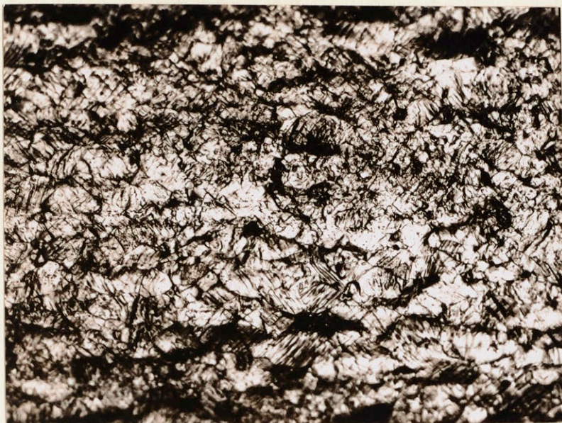
Figure 71. Specimen No. 204 (Point No. 1 of Figure 70). 2S aluminum 500° F, 0.11 hour rupture time. R.A. = 26 percent. 150 x.
