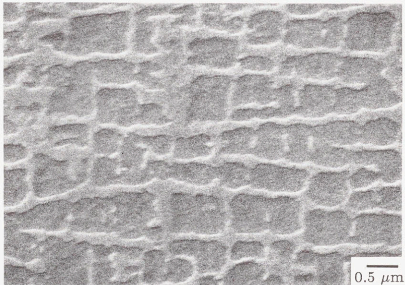
Figure 6.3 Precipitate morphology in CMSX-3 after 114 hours of creep at 850°C and 552 MPa. Tension axis is vertical.
