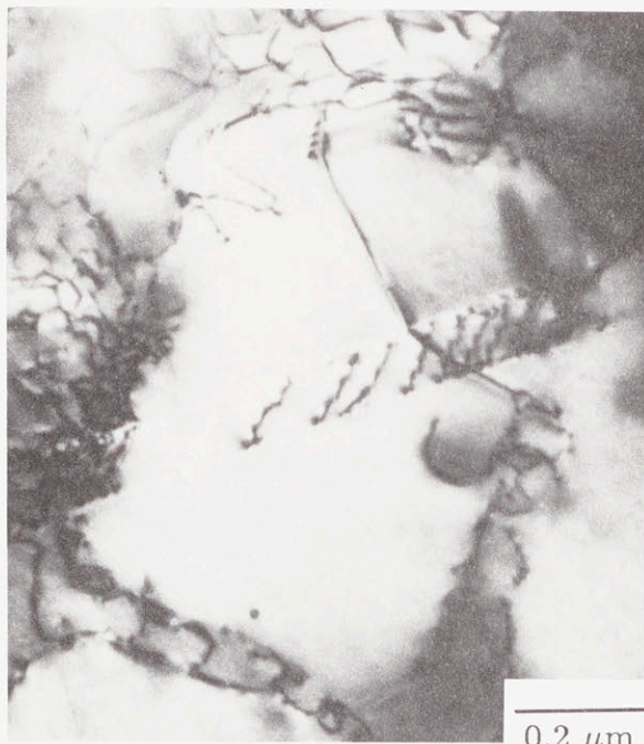
Figure 4.14 A precipitate sheared by dislocations in the later stages of steady state creep.
